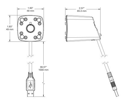
Series 3000 Handheld Sensor Micro USB (DWH200-W):
