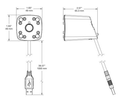
Series 3000 Handheld Sensor Micro USB (DWH200-W):
