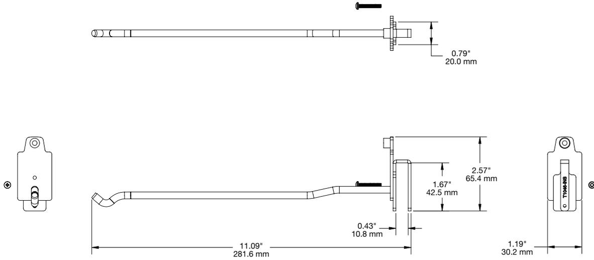
T1000 Rod 12" Slatwall (T1046-S):
