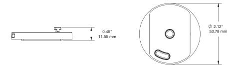
Power Connector, Handheld Micro-USB (CFHM01):
